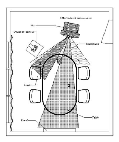
The microphone should be placed at the front of the table to ensure that all speech will be detected. The best position for the microphone is at least 2 meters (6.5 feet) in front of the system on a plain, flat table with at least 0.3 meters (12 inches) of table in front of the microphone.
